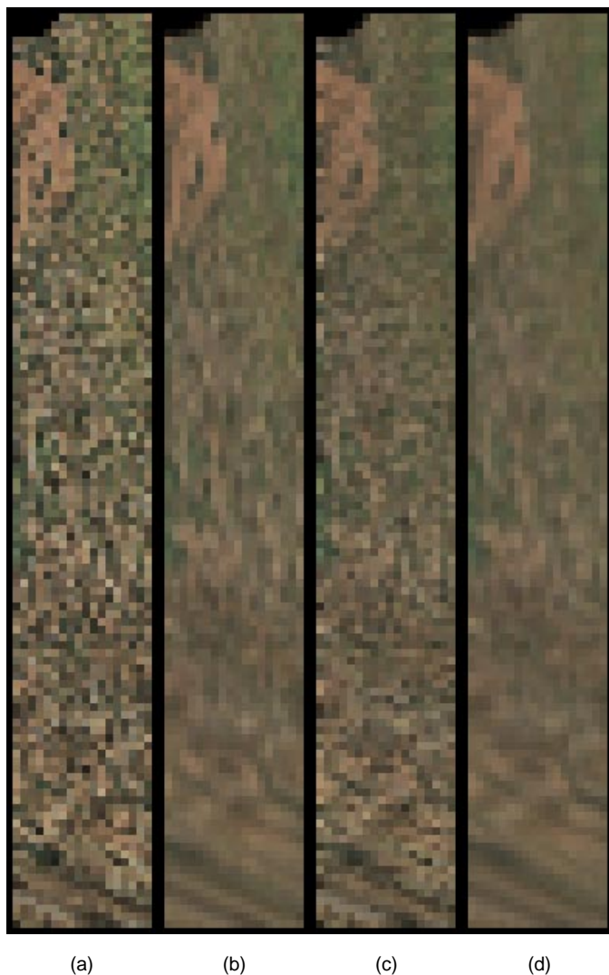
Fig. 14. Animated sequence of the terrain dataset in Fig. 13. (a) Sequence from aliased animation. (b) Sequence from antialiased animation. (c) Sequence from motion-blurred animation. (d) Sequence from antialiased, motion-blurred animation.
