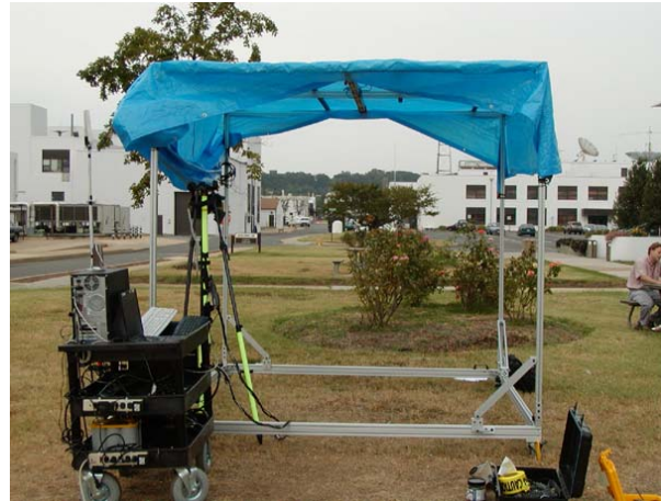
Figure 6. Outdoor tracking cage setup for BARS formative evaluation study. The cage has overhead tracking rails (barely visible under the blue canopy) so that the augmenting graphics can change as a user moves around.
