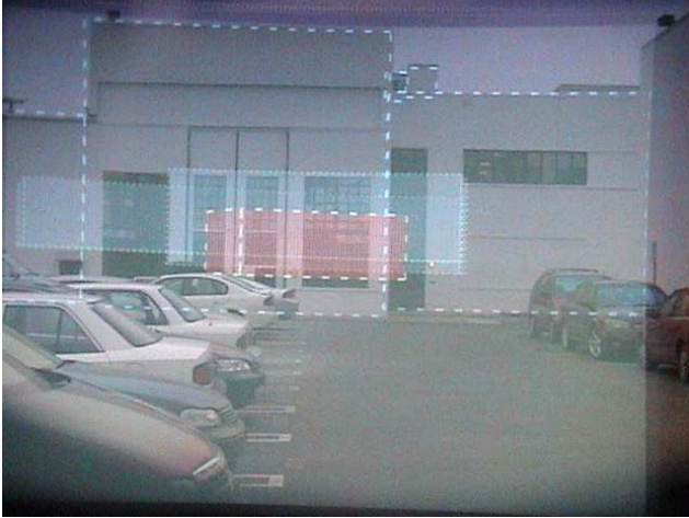
Figure 1. A sample view of our system, showing one physically visible building with representations of three buildings which it occludes.
