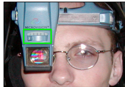
Fig. 2. The experiment used a Microvision Nomad optical see-through AR display. The adjustable focal distance slider is outlined in green.
