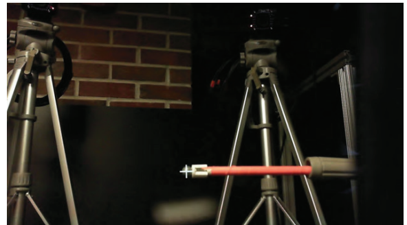
Figure 4: View through the HMD of a control condition alignment, showing the on-screen reticle aligned to the target point.
