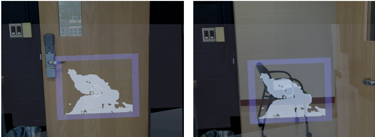
(a) The scanned depth data, as viewed through a closed door.
